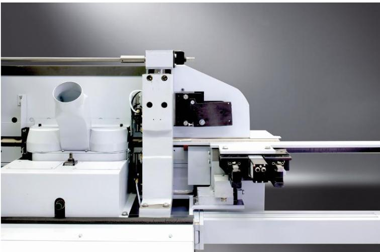
**Fig. 1:** Example of a servo axis, shown here adjusting an infeed fence
