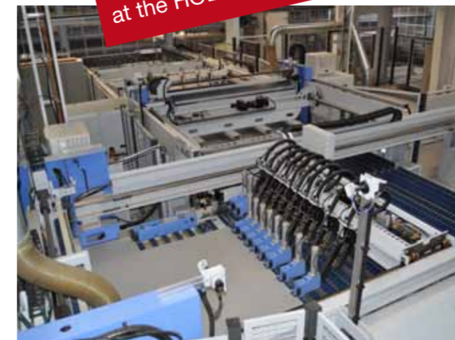
The HOLZMA HKL 380 combiLine is an angular system, which has a routing unit on the rip saw and faster throughput at the crosscut saw thanks to the Power Concept (an additional, variable clamp).
