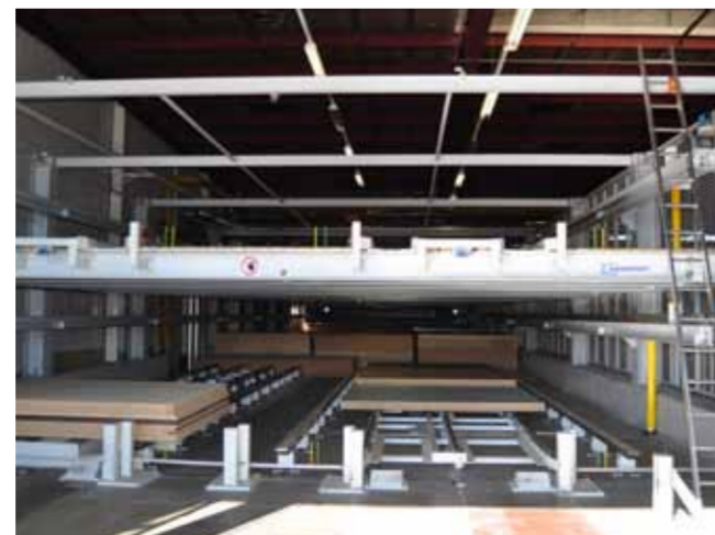
The two-level panel storage system from BARGSTEDT allows access to twice the number of storage spaces and thus reduces access time for the various panel decors.
