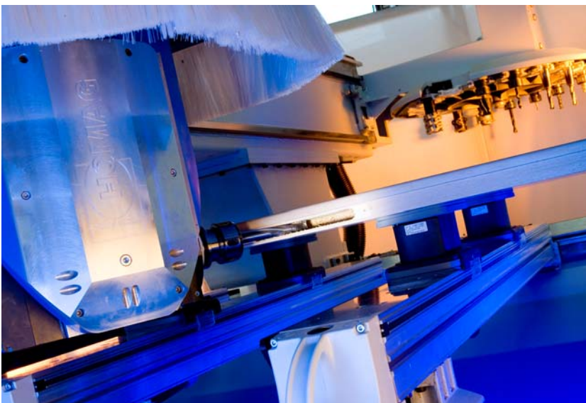
Fig. 4: Lock case trimming with DRIVE5+ five-axis trimming spindle
