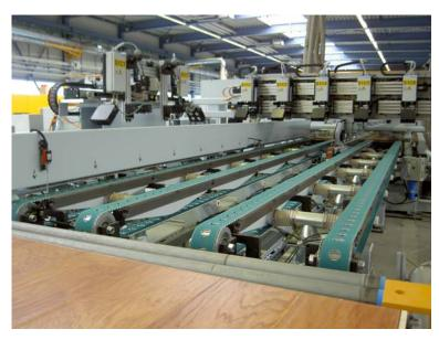
**Fig. 1:** Alignment station with camera gantry
