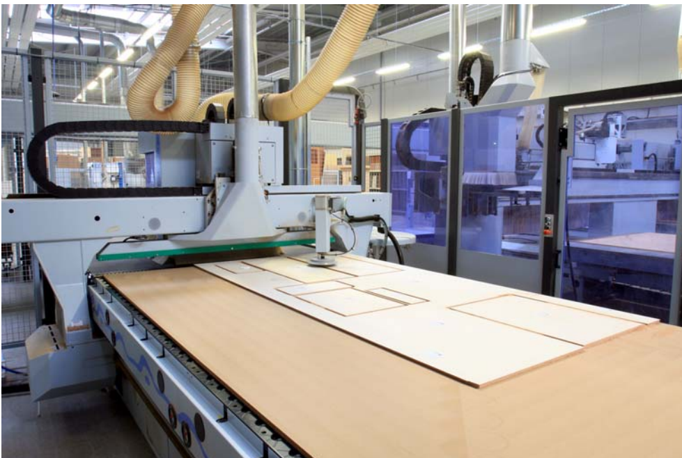
Fig. 4: Cell 2 WEEKE processing centre for automatic and manual infeed
