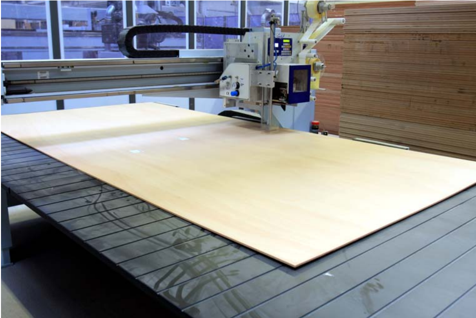
Fig. 5: Labelling of large-format panel prior to nesting
