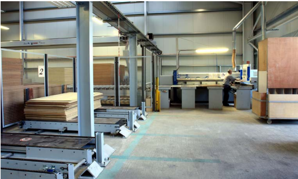
Fig. 2: Existing HOLZMA pressure beam saw integrated into the area storage system
