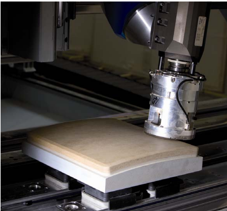
Fig. 2: Traced trimming of curved furniture fronts with DRIVE5C+ five-axis spindle
