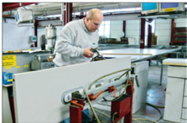
**The stop profiles specially designed by Meta to surround the door thickness are applied using special adhesive**
