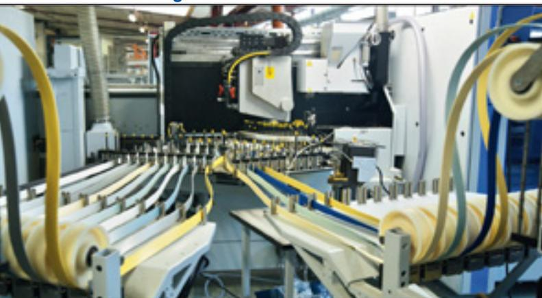
**The laserTec plant melts the PP edge bands onto the narrow side of the panel for a „jointless“ finish using a laser beam**
