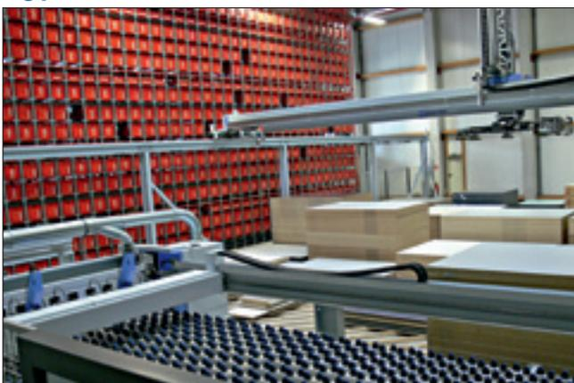
The panels are transported on an order-specific basis from unfinished panel store to the fully automatic production line
