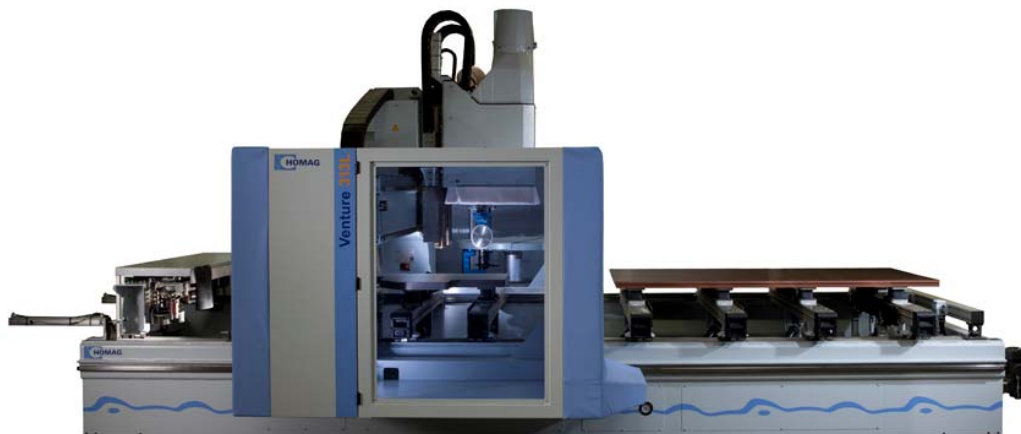
Fig. 2: HOMAG Venture 313 with easyEdge unit
