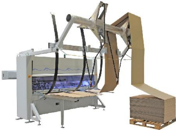
Photo 3: Combination cardboard feeder for individual sheets and continuous cardboard provides even more flexibility for the VKS 200
