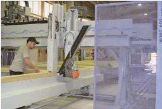
Picture no. 2: Automated frame work generation with the compact PLUS
