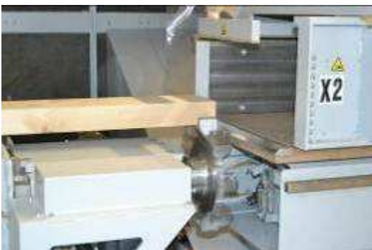
Picture no. 1: Performing notches by means of the underfloor unit
