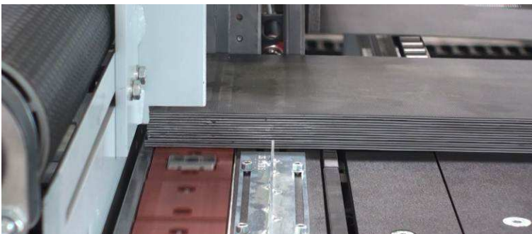
Fig. 3: Vacuum-powered holding-down system and special cams for reliable separation of luxury vinyl tiles.
