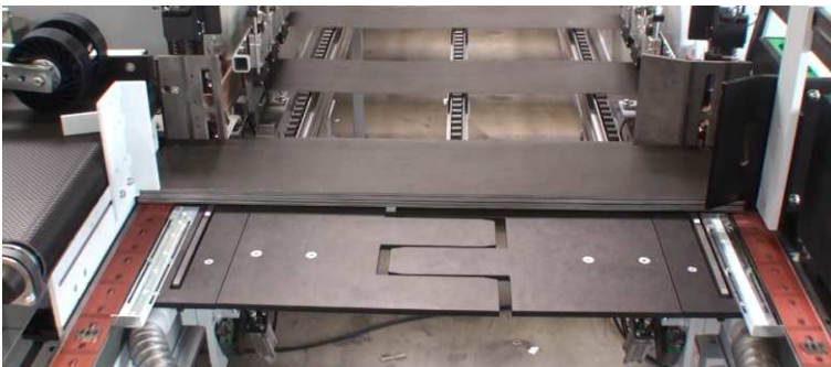
Fig. 2: Magazine in transverse double-end tenoner with table support for LVT
