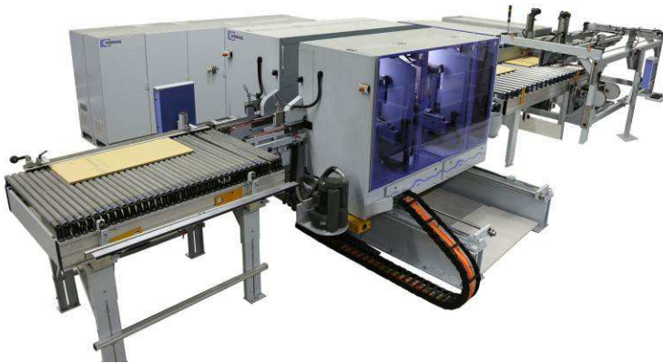
Fig. 4: Angular plant with HOMAG double-end tenoners for profiling wood fiberboard panels
