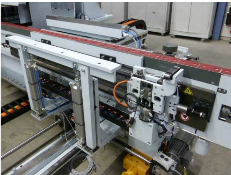
Fig. 8: Vertical pneumatic lifting rail and servo pusher cams at the transverse double-end tenoner infeed
