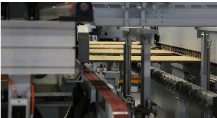
Fig. 6: Angular transfer on two levels with hinging rails for wood fiberboard panels
