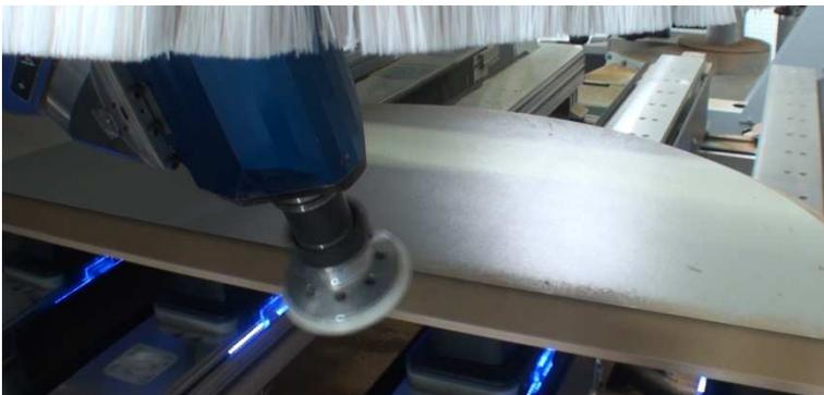
**Fig. 5a:** Finish sanding a chamfer on a table top
