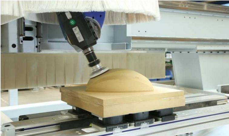
**Fig. 1:** Leveling trimming marks left on a shaped MDF component
