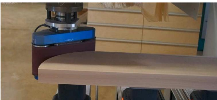
**Fig. 3:** Finish sanding edges using the belt sanding unit
