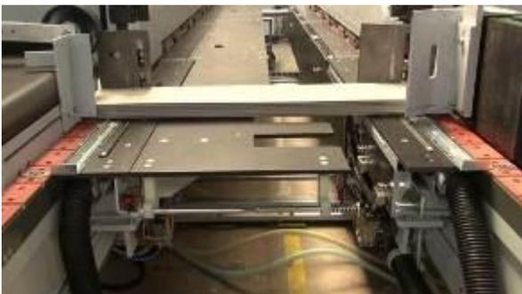
**Fig. 3:** LVT magazine with surface contact tables upstream from cross profiling
