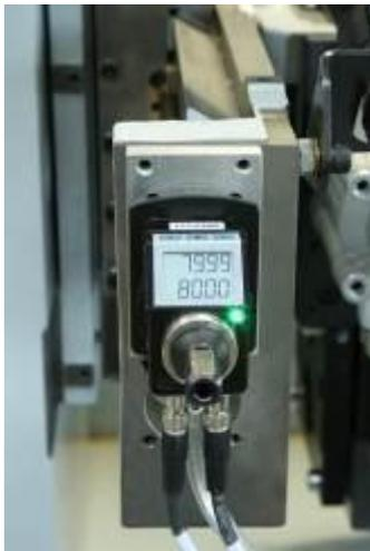
**Fig. 6:** Digital position display at the trimming unit
