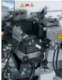
Gluing unit and magazine Coil and automatic strip magazine for a reliable edgmaterial supply. Optimal glue joints, by controlling the exact amount of glue.
