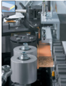
Pressure zone Heavy pressure zone up to 3 mm edge thickness and 50 mm workpiece height for an optimal glue joint (optional 6 mm edge thickness by 60 mm workpiece height).
