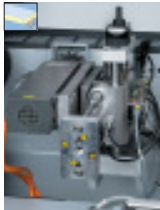
Grooving unit For grooving of drawers or back walls.
