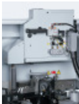
Pre-melter (optional) On-demand availability and perfect glue quality with Quickmelt.
