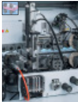
Corner rounding unit Optimum corner rounding without adjustment or set-up, resulting from the coupled DIA tool and tracer roller.
