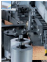
Pressure zone Heavy pressure zone up to 8mm edge thickness and 60mm workpiece height for an optimal glue joint.
