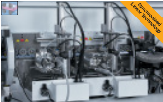
Multifunctional trimming unit (Ambition 1440 FC) Trimming of the edge overhang on top and bottom side as well as contour trimming on the front and rear edges. Equipped with an automatic adjustment to switch between thick and thin edges. Workpiece thickness up to 60mm.
