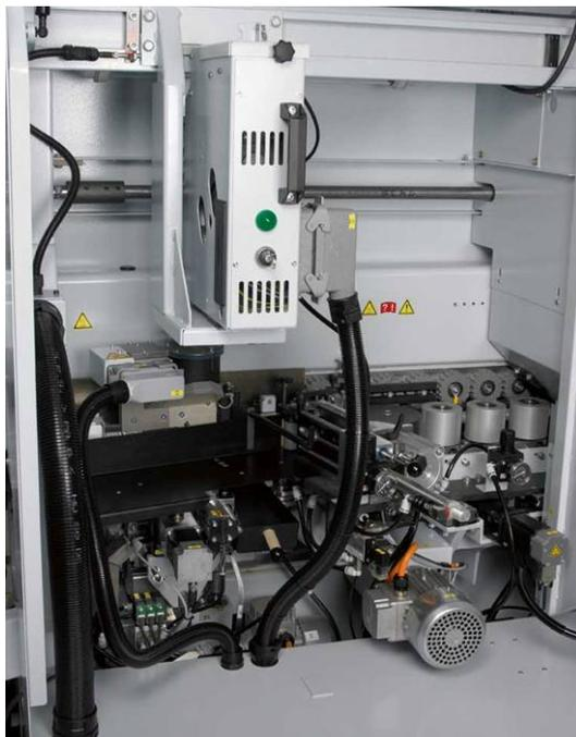
All the functions of the QA 45 are selected using the PC 20+ control system: Metering the glue application quantity, display of maintenance intervals, changing the glue application from synchronous to counter-rotation, or initiation of the cleaning mechanism. Integration of the control system in the machine processes simplifies operation and guarantees even better reproducibility of results – even when changing between operators.
