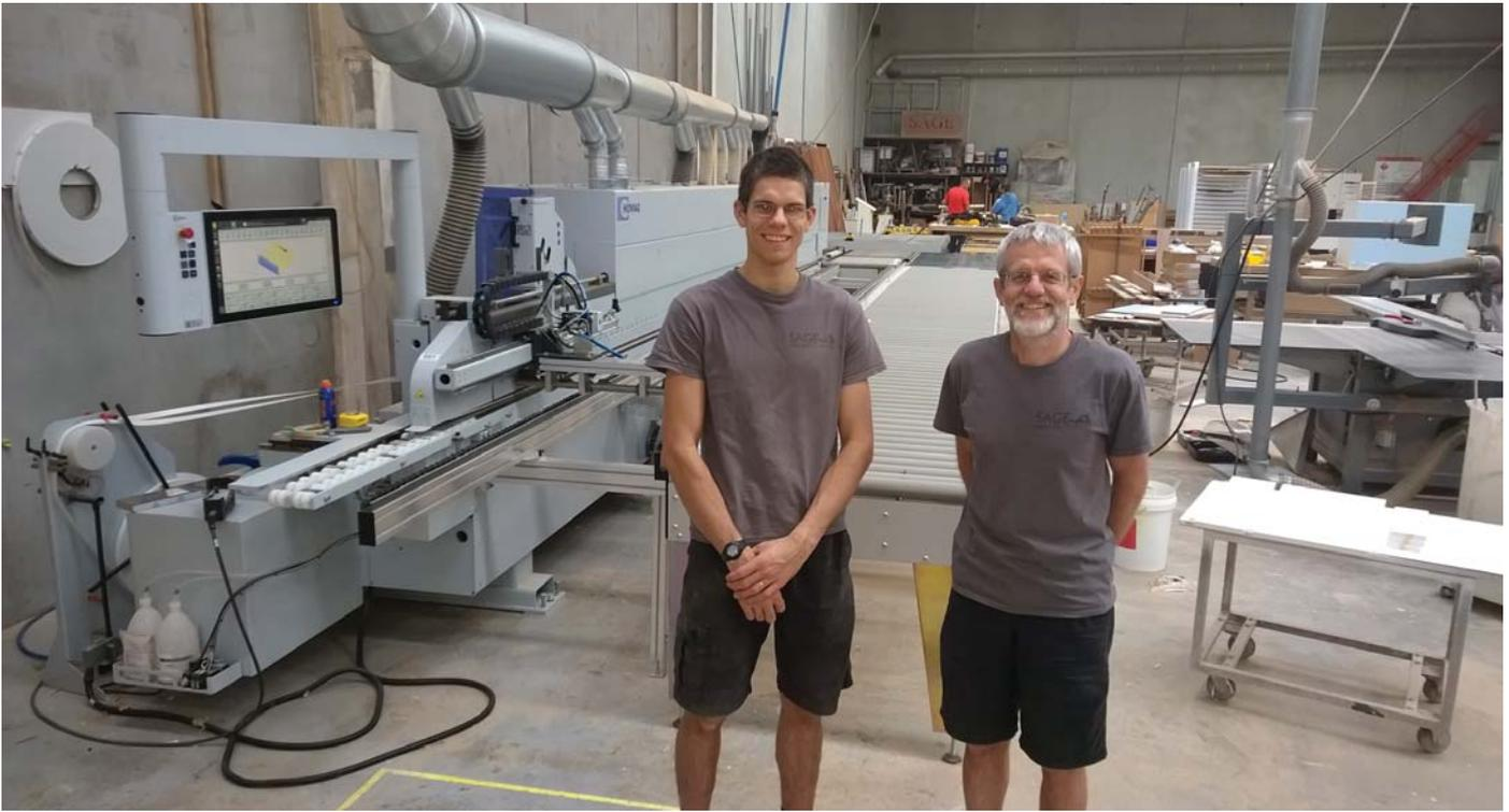
Sage owner John Posthuma and son Michael appreciate the latest addition to their manufacturing process: a hot-air enabled edgebander from Homag which is capable of working with laser-edged tape. Together with the Weeke Vantage 100 cell the Auckland based company have stepped up massively in their production capacity.
