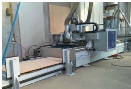
The Homag Group's airTec is a simple technology where the function layer on the edging material is reactivated by compressed hot air. Alexis Pantelides, Homag New Zealand's sales representative, explains, “The work piece thickness is adjustable with a pusher in the compressed air nozzle and it is simple to change between hot melt and airTec.”
