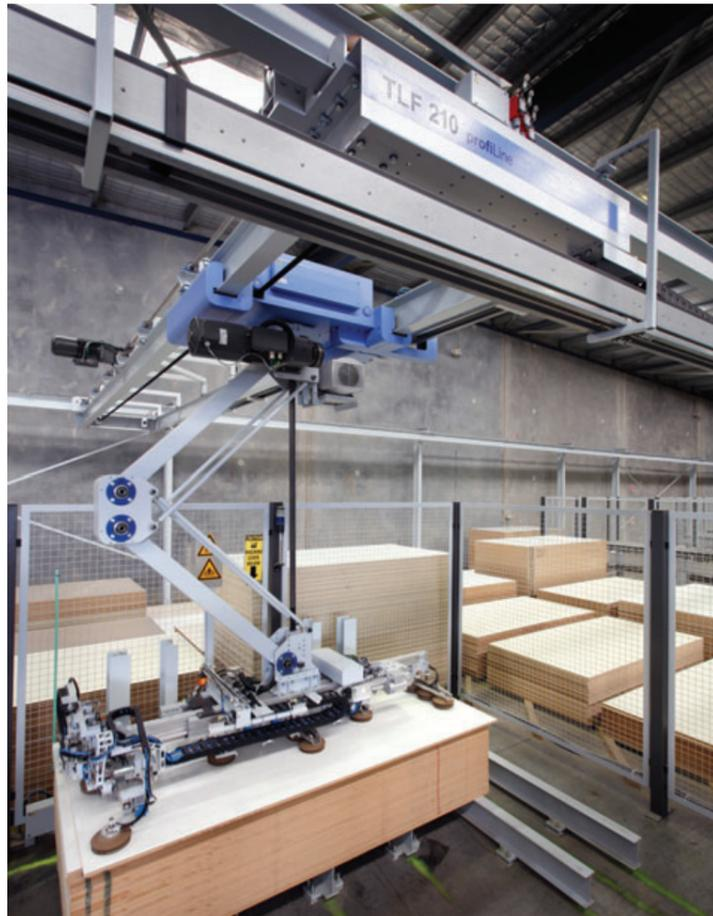
With Homag technology, the manufacturing process ensures minimal waste of raw materials. The Bargstedt TLF 210 feeds the sheets directly to the Weeke nesting cells and the Holzma beam saw.
