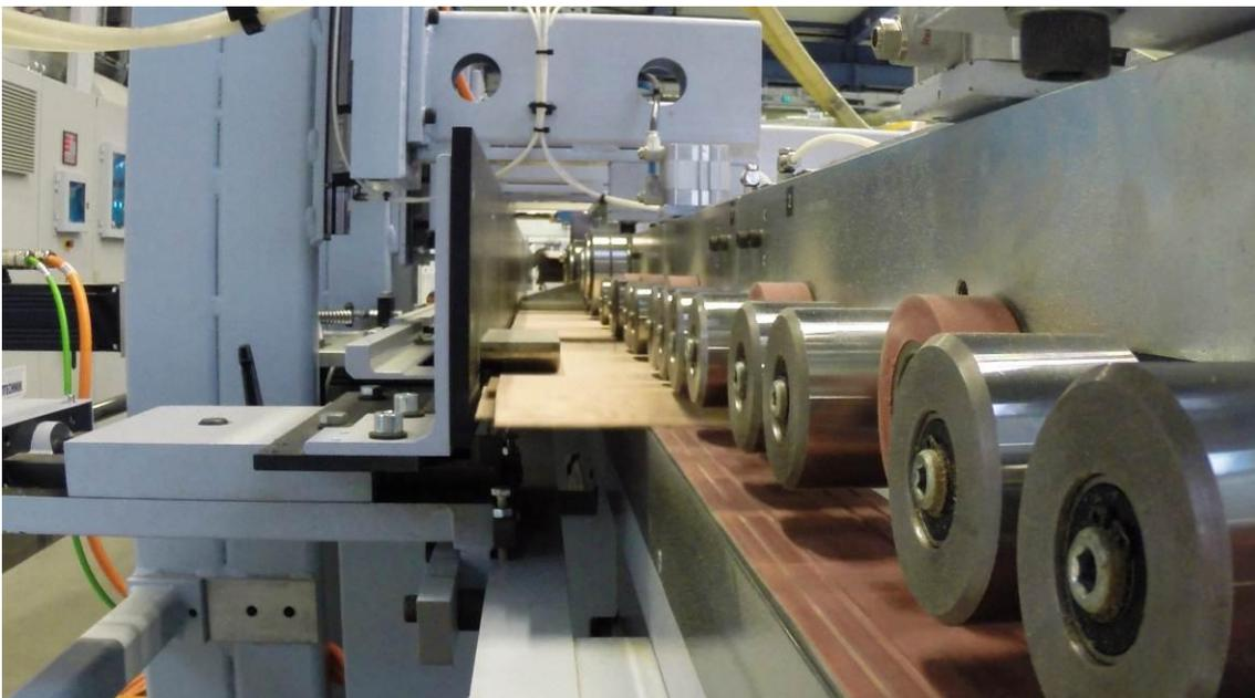
**Figure 4:** Alignment guide of the longitudinal machine
