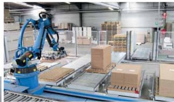
At Recor, 3 robots are palletizing and thus care for an automatic panel flow from delivery to labeled packages
