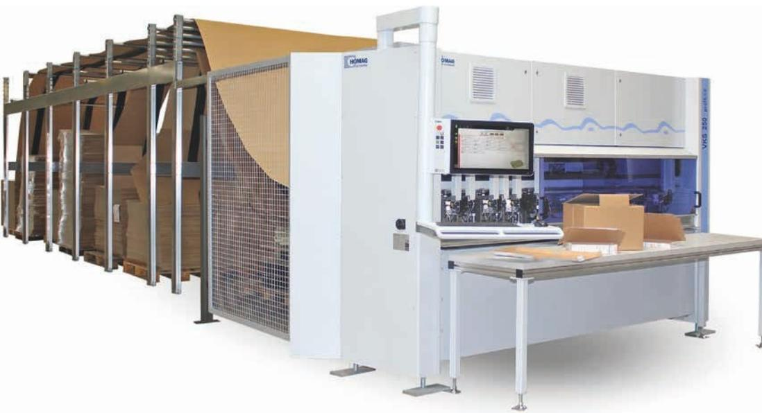
(right) Example of a cardboard cutting machine type VKS 250
