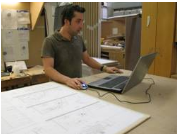
The parts list is created in the hall: The employee responsible for the order fetches one of the laptops, creates the parts list based on the plan and sends it
