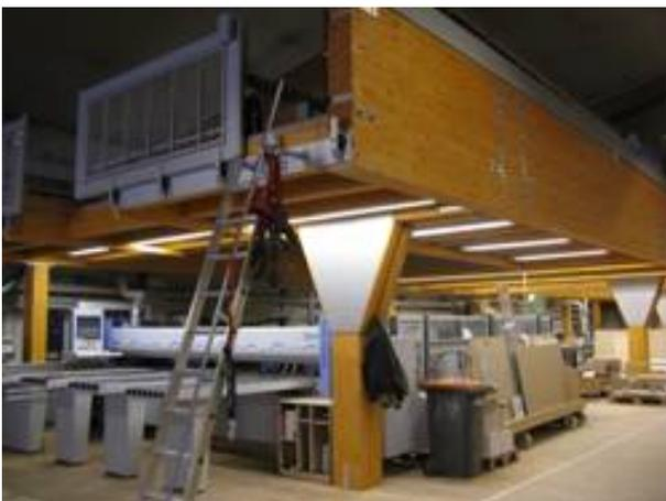
Above the saw is the intermediate level: the proprietary wooden construction accommodates the 30 x 8 m BARGSTEDT TLF 410 storage system with 15 positions and an advance stacking position. This created 275 m<sup>2</sup> of additional working area on the ground.
