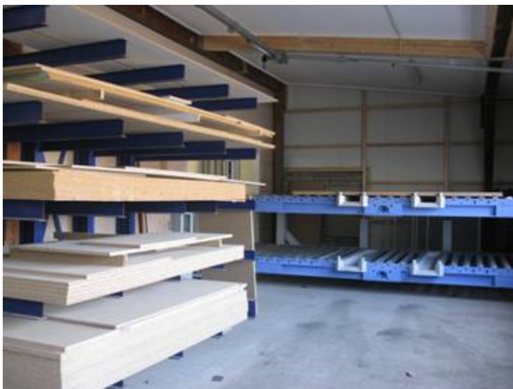
Picture 6: Additional two-level roller conveyor leading directly from the warehouse to the saw's lift table
