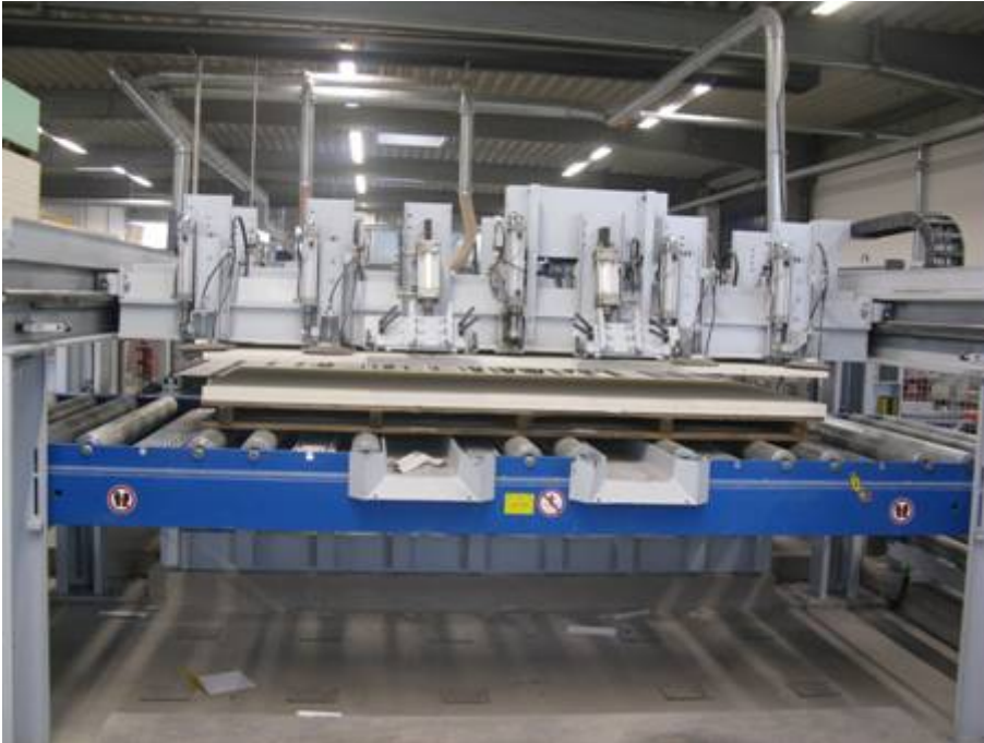
Photo 3: A single panel is moved from the lift table to the rear machine table using vacuum suction cups.
