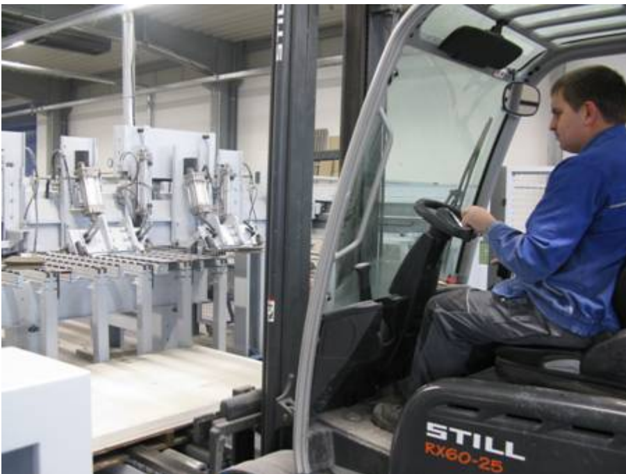
Photo 2: The saw is fed with a stack of panels via the lift table. Panels are then transported through the saw fully automatically.
