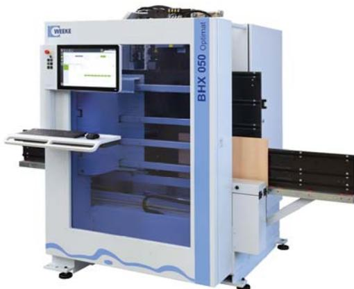
“From nesting, they go either to the WEEKE BHX 050 drilling centre or direct to the new BRANDT Highflex 1230 edgebander. Again, the speed, accuracy and finish quality from both these machines is just outstanding. Using our old edgebander we had to hand finish every
