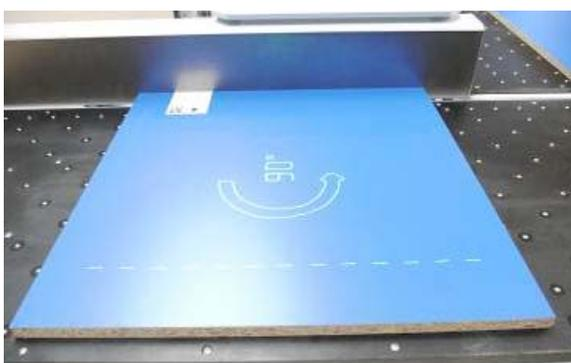
**The HOLZMA system guides the machine operator visually – for example by means of laser projections on the workpiece**
