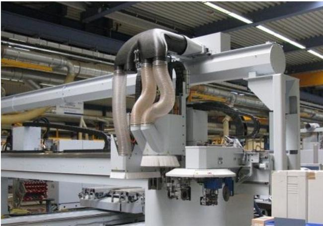
**The new flow-optimized CFK distributor on HOMAG CNC-machines**
