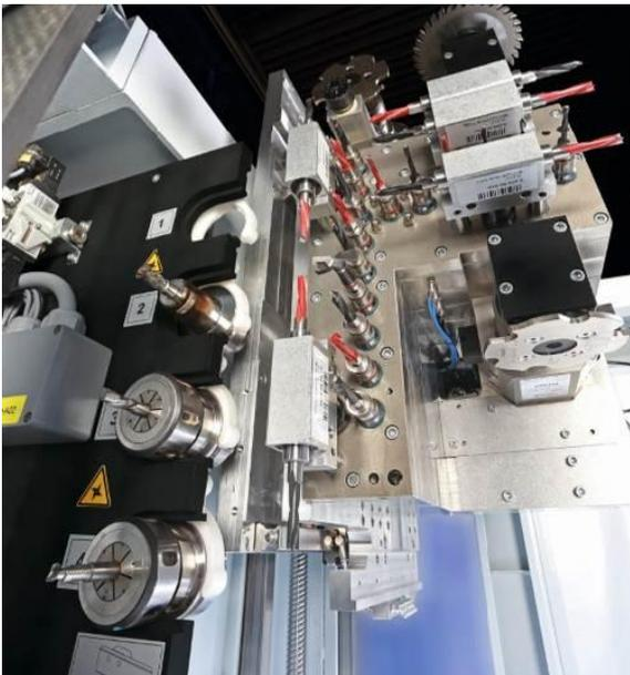
**Vertical processing centre of WEEKE: One single drilling block with 25 high speed drilling spindles.**
