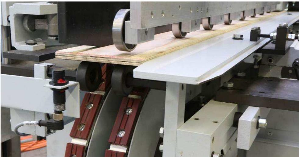
**Fig. 4:** Entry into double-sided profiling: the rolling chain provides a high level of processing accuracy and a long service life
