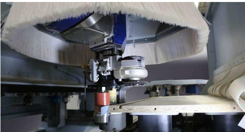
**Fig. 5:** The patented **easyEdge**: Edge banding using the DRIVE5C+ 5-axis spindle
