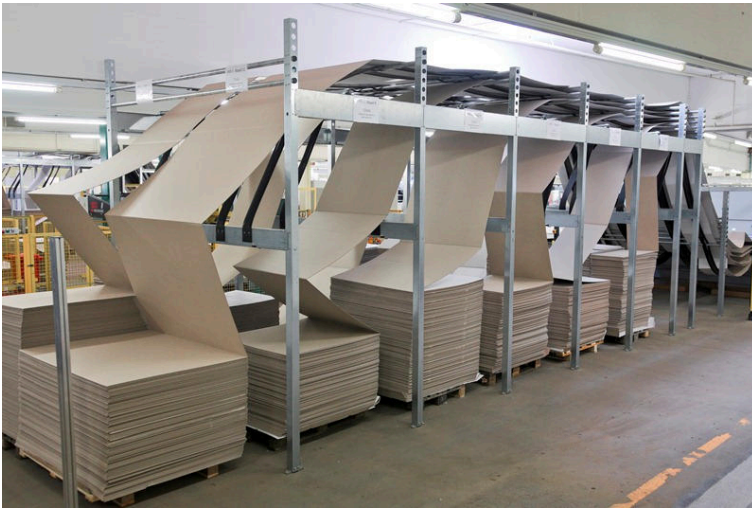
Picture 5: VKS 250 powerTouch with sixfold endless cardboard change system and side-by-side function. This enables an optimal, automatic packaging out of 12 different web widths.
