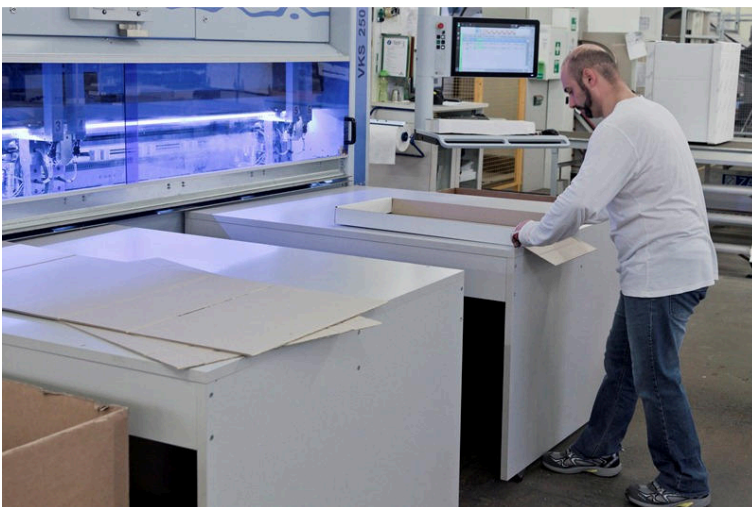
Picture 6: The VKS 250 powerTouch automatically produces the proper cutting for every cupboard, as individually as it is.
