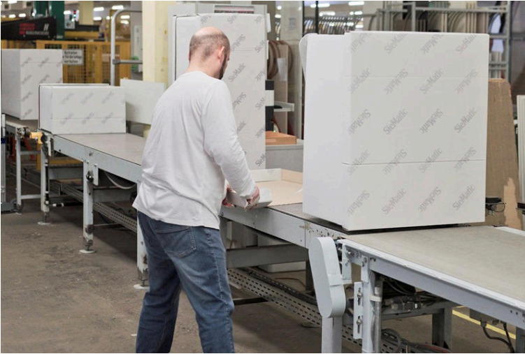
Picture 7: Afterwards, the final assemblies corpuses are packed on the transport line and prepared for delivery.
