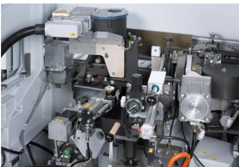
Picture 3: BRANDT - Gluing unit QA 45 with short heat up time and rapid glue type changeover.
