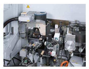
**Picture 2:**Glue application system QA 45 with a short heating-up time and quick retrofit facilities
