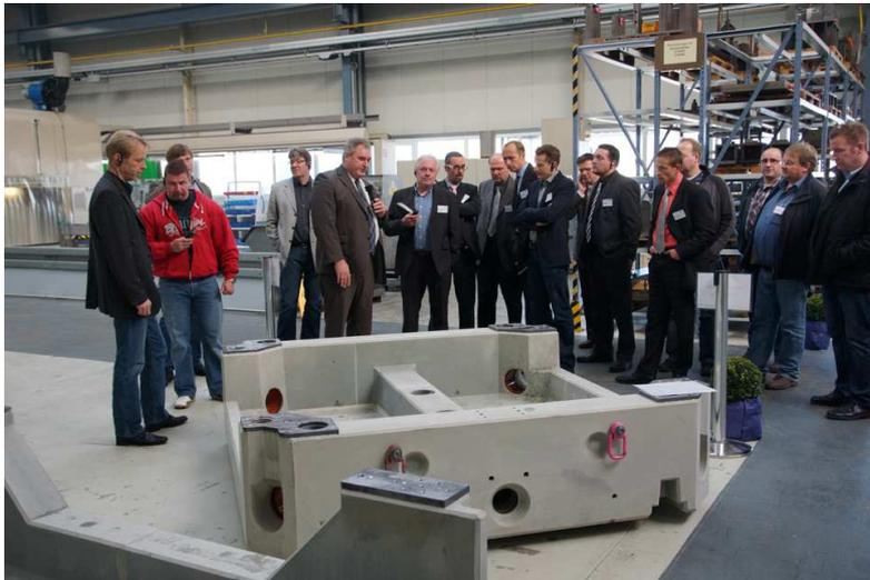
**Pic:** Tour of the production hall to inspect the BÜTFERING sanders; shown here is a machine bed made of the vibration-absorbing material SORB TECH.
