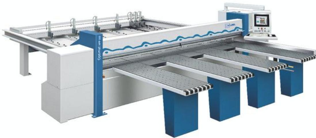
"At first glance, this technical redesign is easy to overlook, but is noticeable as soon as you see the speed and cutting quality. The range has an entirely new saw carriage design; the designers, however, have maintained the low working height of the air tables at the ideal ergonomic height of 920 mm - this minimises bending thus protecting the back of the operators.
