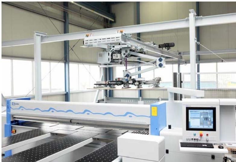
Simon Brooks, sales and marketing director for Homag UK takes up the story, "Not only does IntelliStore reduce the floor area that is required for stock, but it also improves the yield from the saw because it is the software that controls the output from the device, rather than having to rely on the operator to keep feeding the machine at the optimum rate.
