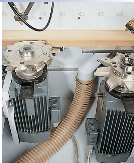
Smoothing / radius trimming Trimming the chipboard down to laminate thickness and rough radius trimming from below.
