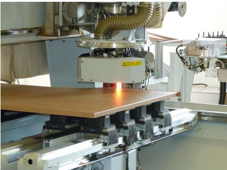
**Fig. 4:** The freeform sides of the furniture components are also given laser edges at the processing centers.
