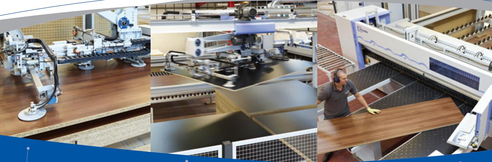
The crane automatically selects and picks up the correct board from stock
