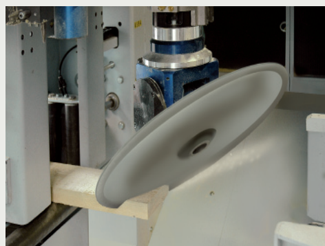
Universal tool spindle for the application of various tools and the generation of all required connections for timber house construction
