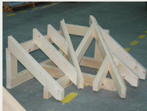
Flexible beam processing for the production of component parts for timber frame houses and roof constructions
