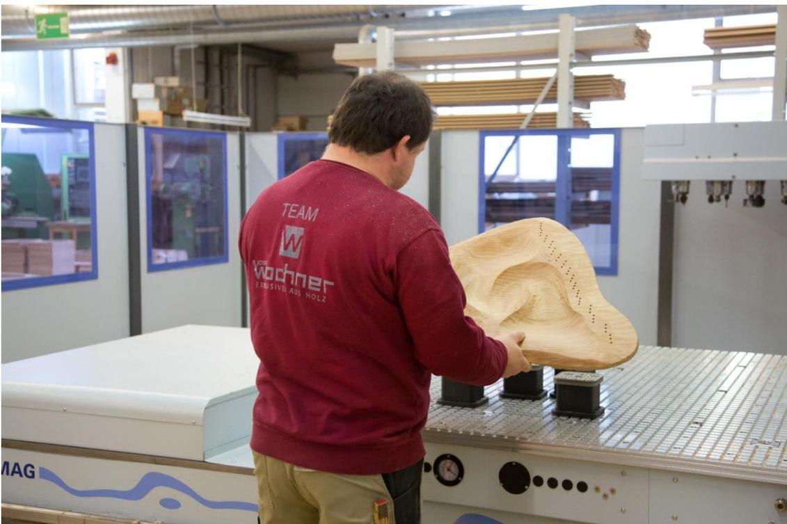
**Figure 2:** HOMAG has created the 3D model with the scanner and Wochner has used this model to generate a CNC program with Alphacam and has trimmed the reproduction.
