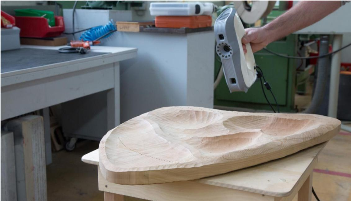
**Figure 1:** A specialist at HOMAG guides a hand scanner around a piece of art and creates a 3D model for reproduction on the CNC.
