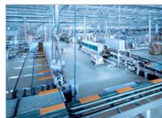
Flexible sizing and edge processing line from HOMAG with feed and stacking station from BARGSTEDT
