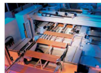
WEEKE drilling line with feed and stacking station from BARGSTEDT
