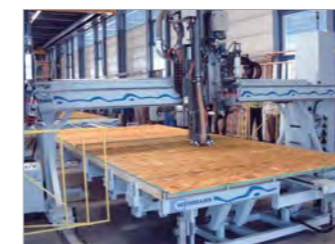
Multifunction bridge for processing prefabricated house elements from WEINMANN
