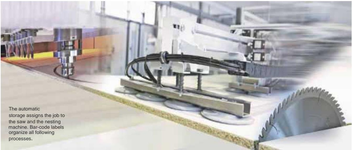
The automatic storage assigns the job to the saw and the nesting machine. Bar-code labels organize all following processes.
