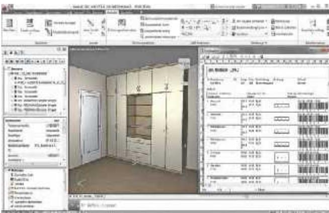
WoodCad/Cam provides CNC programs, Cut-Profi(t) the layouts.
